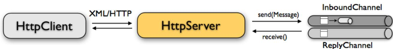
The figure above shows the basic setup with inbound channel and reply channel. You as a tester should not worry about this too much. By default, you as a tester just use the server as synchronous endpoint in your test case. This means that you simply receive a message from the server and send a response back.
