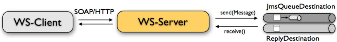
The figure above shows the basic setup with inbound channel and reply channel. You as a tester should not worry about this to much. By default you as a tester just use the server as synchronous endpoint in your test case. This means that you simply receive a message from the server and send a response back.
