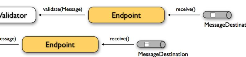
The message receiving component passes the message to the validator where the individual validation steps are performed. Let us have a closer look at the validation options and features step by step.
