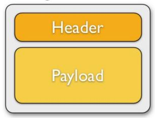
A message consists of a message header (name-value pairs) and a message payload. Later in this section we will see different ways of constructing a message with payload and header values. But first of all let's concentrate on a simple sending message action inside a test case.
