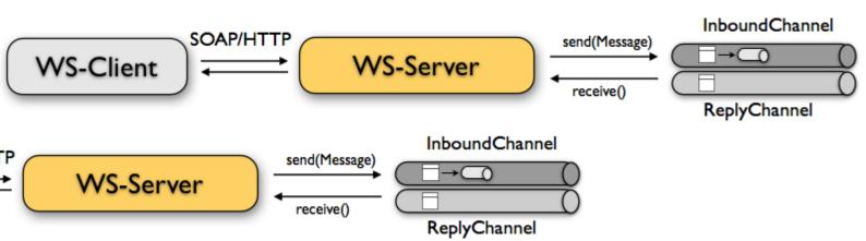
The endpoint works together with the message endpoint adapter that is responsible for providing a response message for the client. The various message endpoint adapter implementations in Citrus were already discussed in endpoint-adapter.
