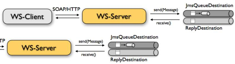
The figure above shows the basic setup with inbound channel and reply channel. You as a tester should not worry about this to much. By default you as a tester just use the server as synchronous endpoint in your test case. This means that you simply receive a message from the server and send a response back.
