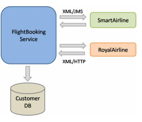
In our example two different airlines are connected to the FlightBookingService application: the SmartAriline over JMS and the RoyalAirline over Http.
