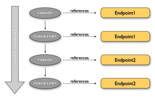
The figure above describes a typical test action sequence in Citrus. A list of sending and receiving test actions composing a typical test case here. Each action references a predefined Citrus endpoint component that we are going to talk about later on.
