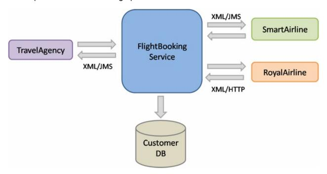
In our example two different airlines are connected to the FlightBookingService application: the SmartAriline over JMS and the RoyalAirline over Http.
